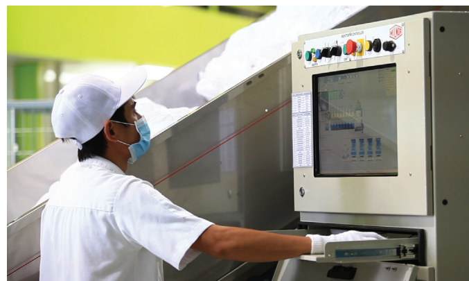
INSIDE VIEW: Milnor's Mentor® controller allows operators to see the progress of batches within the tunnel
