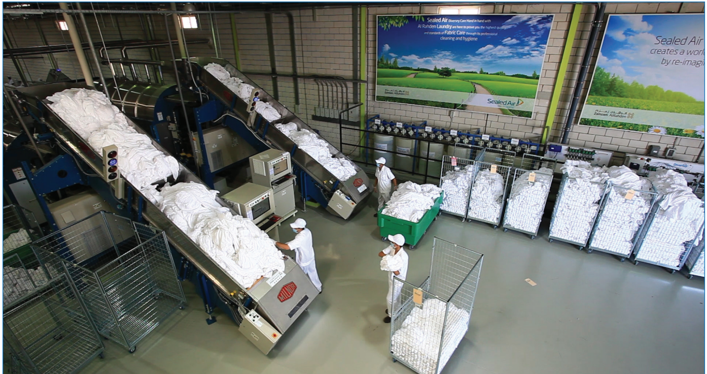
LOADING THE TUNNELS: AlRahden has two PBW™ tunnel lines, one based on the 50kg, five-module 76028 used mainly for garments, and the other on the 76039 (left in picture) a 68kg, eight-module machine for bed linen
