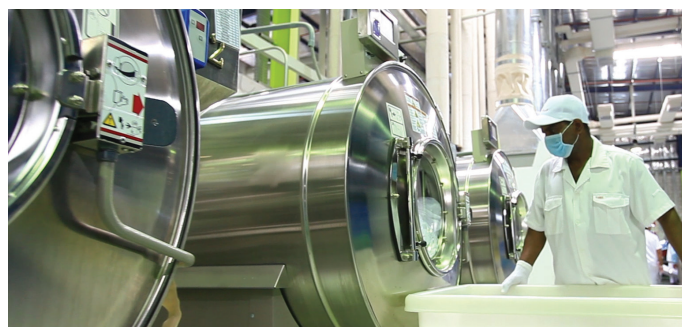
EFFICIENT WASHER-EXTRACTORS: AlRahden's Zamzam laundry uses 42030 V6Z washers with Milnor's RinSave® water saver which reduces the number of rinses needed by using precise high G-force to "sling" the wash liquor after the last wash stage
