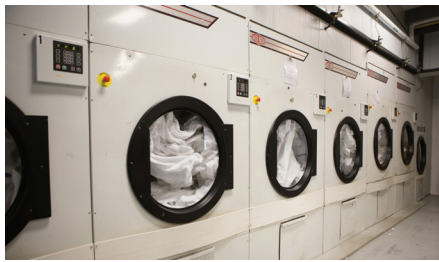
NO CONTEST: Choosing Milnor equipment for Superior Laundry's new facility was a simple decision – especially after salvaging two 86kg (190 lb) Milnor dryers pictured second and third from the right.
