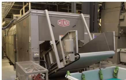
CENTRIFUGAL POWER: Added post-fire, Milnor's centrifugal extractor helps remove excess water from linens in Superior Laundry's new facility.
