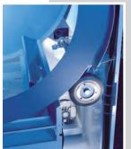
Some dryers use the same type of drive and support as 400 lb. dryers. There's no maintenanceprone gear box either. (Feature available on M96, M122, M175, M190 and M202.1
