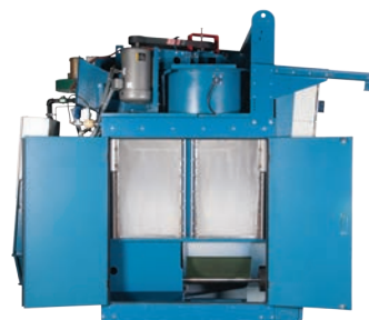
Milnor's 6464 internal lint filter has 11.41 ft 2 surface area.
