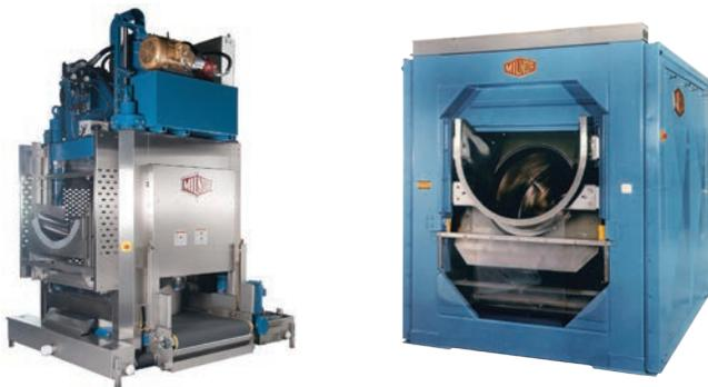
*Various capacity sizes and extraction pressures and speeds are available in the Single Stage Press and Centrifugal Extractor. Other options are available for tight spaces.*
