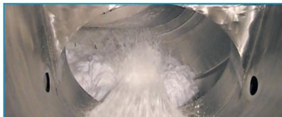
*This feature in the first module of each PBW washer is a patented pump arrangement which quickly wets down the goods. Additionally, this recirculated water adds a hydraulic effect which speeds up the cleaning action of the chemistry.*
