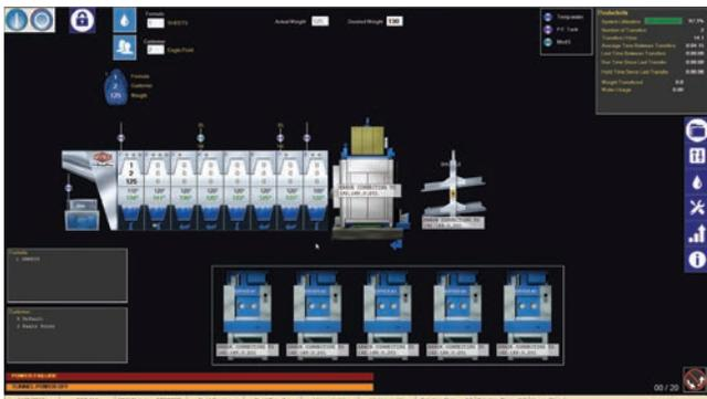
*The operational display gives key information for each batch in the loading system, washer and post-washing devices.*
