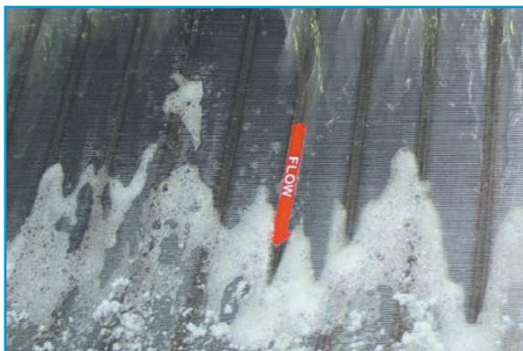
*The 430 micron wedgewire screen removes lint and other solids from the process water.*
