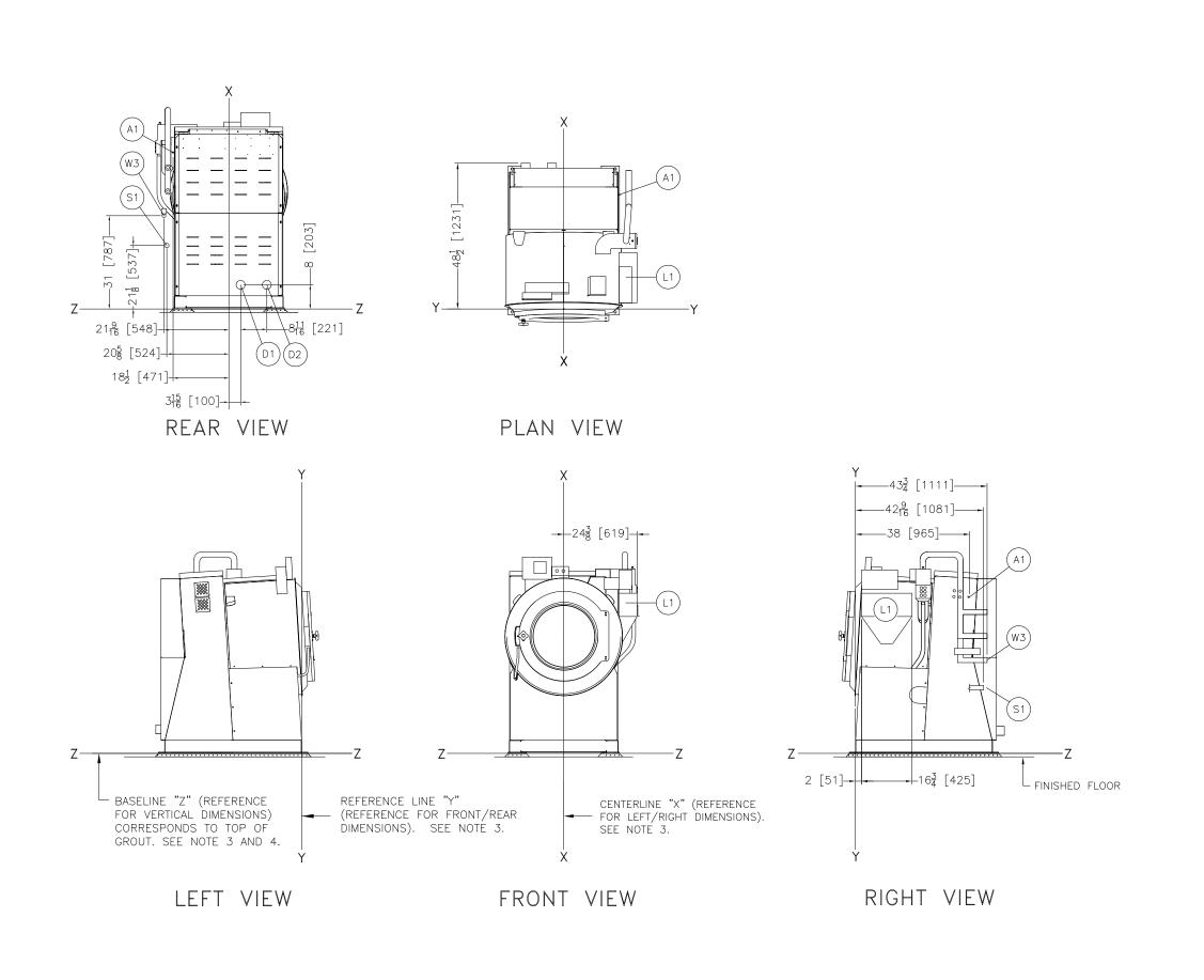
W3 REUSE INLET (AIR OPERATED), 1-1/4" NPT CONNECTION STEAM, 3/4" NPT (AIR OPERATED) COMPARTMENT SUPPLY DUAL DRAIN, DRAIN TO SEWER, 3" PIPE SOCKET JOINT D1 DUAL DRAIN, DRAIN TO REUSE, 3" PIPE SOCKET JOINT. /4" AIR CONNECTION, REQUIRED FOR AIR OPERATED REUSE OR AIR OPERATED STEAM, CUSTOMER MUST SUPPLY AIR
