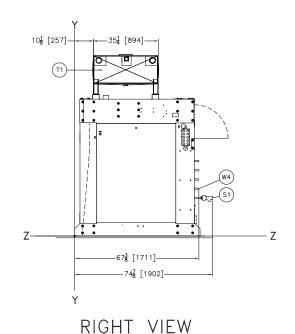
W4 THIRD (OR REUSE) WATER INLET, ELECTRICALLY OPERATED, 3/4" NPT CONNECTION OPTIONAL AIR-OPERATED STEAM INLET, Y-STRAINER REMOVED FOR SHIPPING MUST BE ADDED AT INSTALLATION, 1"NPT CONNECTION T1 OPTIONAL TANK (PIPING NOT SHOWN) 5 COMPARTMENT SUPPLY OPTIONAL SINGLE DRAIN DOWN, 3" PIPE SOCKET JOINT CONNECTION LEGEND
