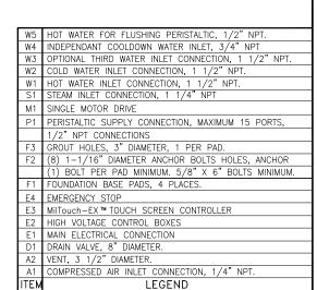
10 SHIM TO LEVEL THE MACHINE AND ALLOW FOR 1" [25] MINIMUM GROUT. ANCHOR WITH ONE ANCHOR BOLT PER PAD, MINIMUM. USE 5/8" X 6" BOLTS, MINIMUM. SEE INSTALLATION MAINTENANCE MANUAL FOR FURTHER INSTRUCTIONS.
