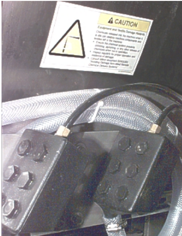
Figure 1: Pumped Chemical Inlets on CBW Batch Washer
