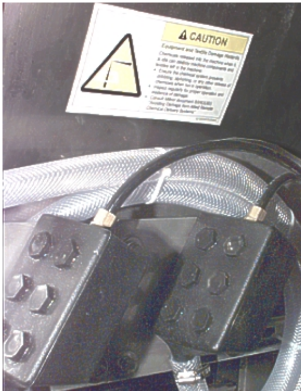
Figure 1: Pumped Chemical Inlets on CBW Batch Washer
