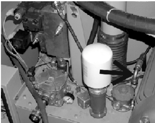
Figure 14: MP1A03 hose connection (L7b) at hydraulic tank filter
