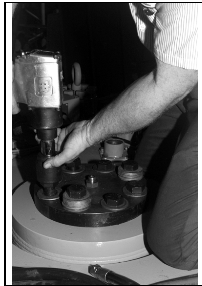
Figure 4: Install Hydraulic Fitting Equipped Cylinder Cover
