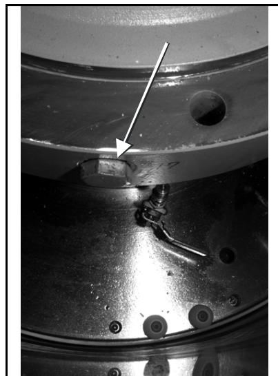
Figure 6: Remove Ram Drain Plug
