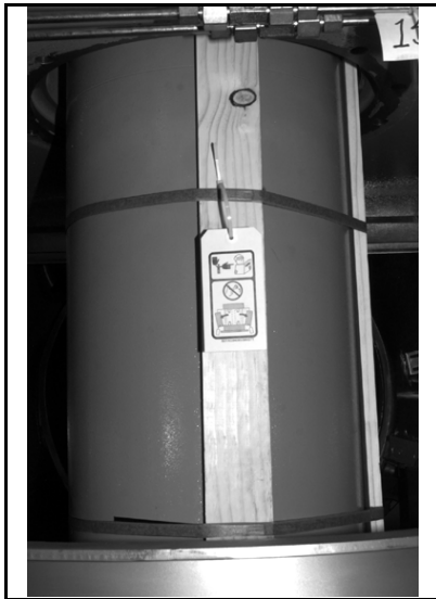
Figure 7: Remove the Cylinder Shipping Material
