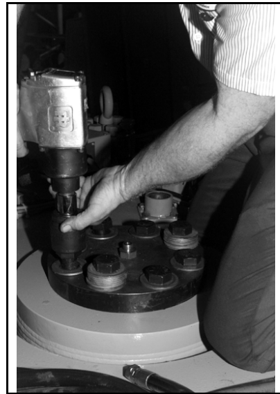
Figure 4: Install Hydraulic Fitting Equipped Cylinder Cover
