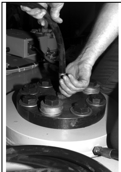
Figure 5: Installing Fill Hose from Pump
