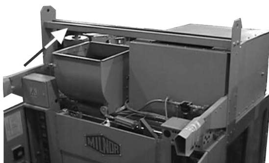
Figure 3. Spreader Bar Between Front Lifting Plates
