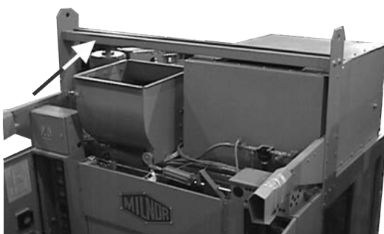
Figure 3. Spreader Bar Between Front Lifting Plates
