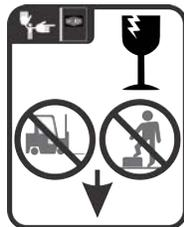
B2TAG94078: Do not forklift here; do not jack here; do not step here—whichever applies.
