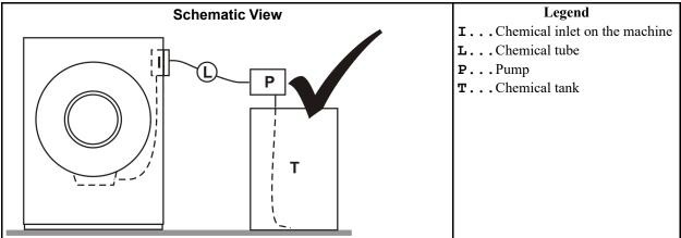
**Prevent leaks.** — When you do maintenance on the chemical pump system:
