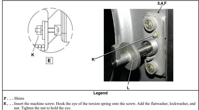
**L**...Put the free end of the spring into this hole.
