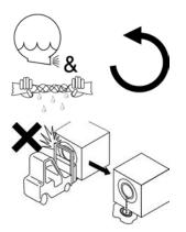
B2TAG94099: Do not strike the shell door when fork-lifting. This can cause the door to leak.
