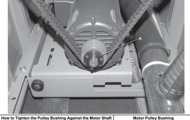
How to Tighten the Pulley Bushing Against the Motor Shaft It is necessary to use both bolt torque and careful hammer blows with a brass or rubber hammer to fully tighten the motor pulley bushing. When the pulley and bushing are installed on the motor shaft and aligned with the main drive pulley, tighten the motor bushing as follows:
