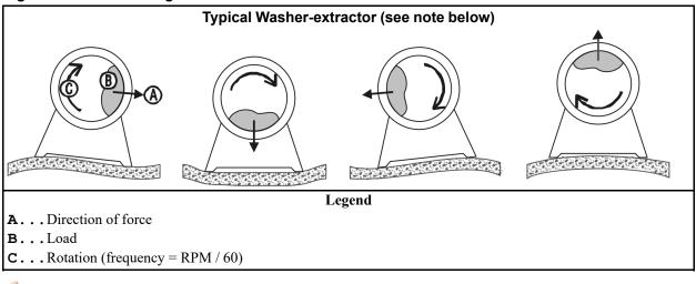
Figure 5. How Rotating Forces Act On the Foundation
