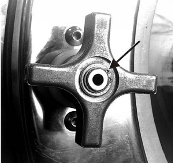
Figure 19. Front Retaining Clip and Thrust Washer
