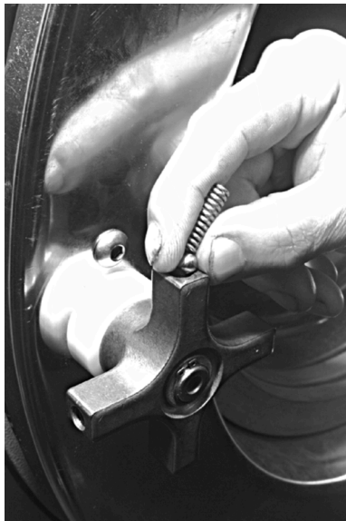
Figure 26. Inserting Ball and Spring in Handle Spoke
