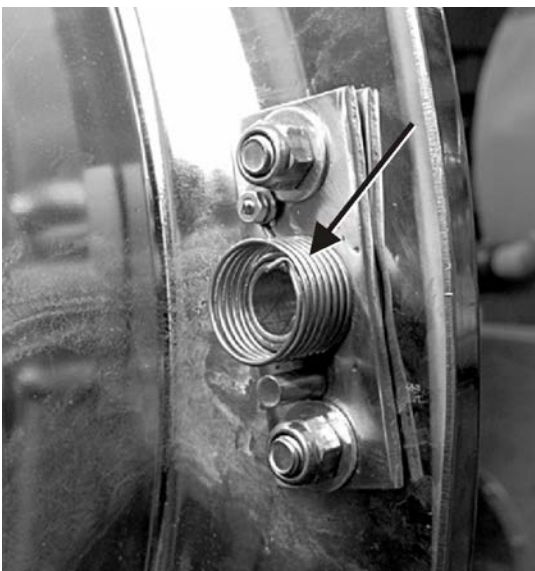
Figure 21. Return Spring After Separation from Shaft Cam
