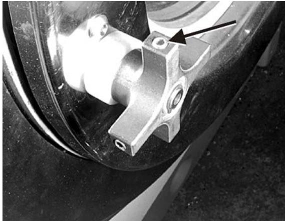
Figure 17. Door Handle Spoke Set Screw
