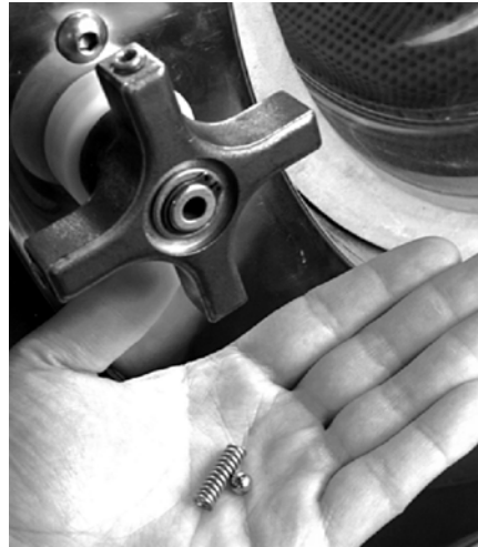
Figure 18. Handle Spoke Spring and Ball
