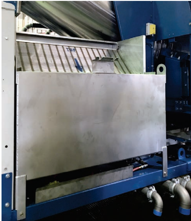
Figure 3: Wedge Wire Sub-assembly
