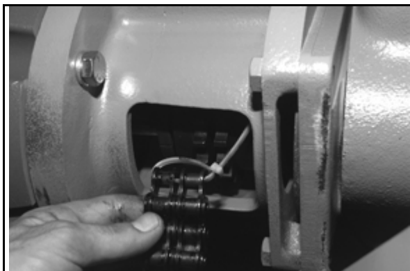
Figure 11: Starting chain into sprockets
