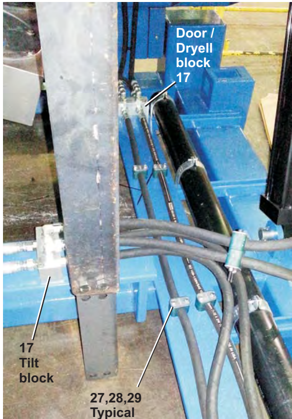
Figure 2: Junction blocks and counterbalance valves
