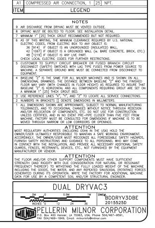
W1 SPRINKLER WATER INLET, 1-1/4"[31] NPT PIPE CONNECTION .406[10] DIAMETER ANCHOR BOLT HOLES. USE 3/8"[10]
