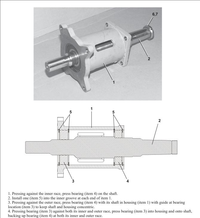
5. Install retaining rings (item 5) into outer grooves.
