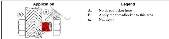
**3.3. Disassembly**—For high-strength threadlocker, apply heat for five minutes. Disassemble with hand tools while the parts are hot.
