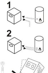
B2TAG94091: Drain the condensate to the sewer during first one hour after commissioning a new machine or replacing the steam coil. This flushes out any residual anti-freeze that might be in the steam coil. After one hour, condensate can be returned to the boiler.
