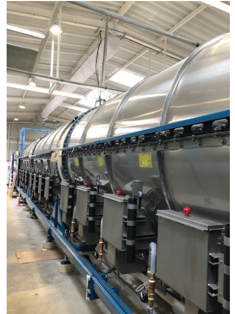
NEW TECHNOLOGY: In addition to its 30-year-old CBW, Gallia operates a new 76039 PBW featuring PulseFlow technology
