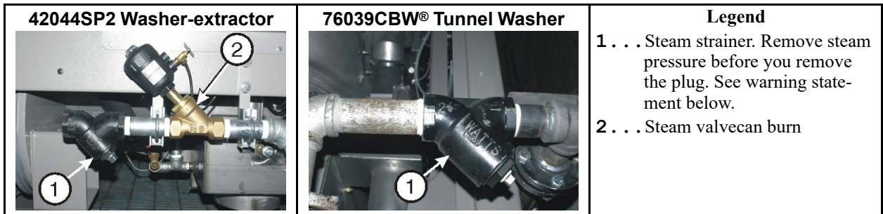
Figure 14. Steam Inlet Strainer. These are examples. Your machine can look different.
