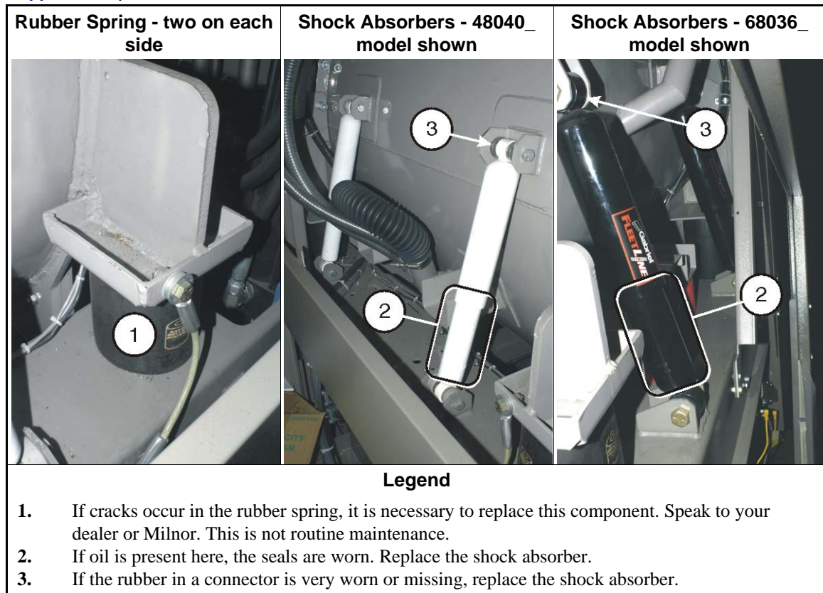
Figure 19: Suspension Components on Each Side of Rubber Spring-resting Washer-extractor (see Supplement 4)
