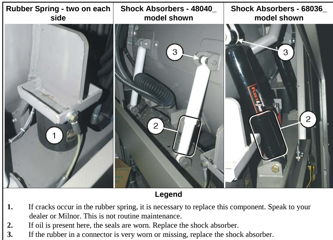
Figure 14: Suspension Components on Each Side of Rubber Spring-resting Washer-extractor (see Supplement 3)
