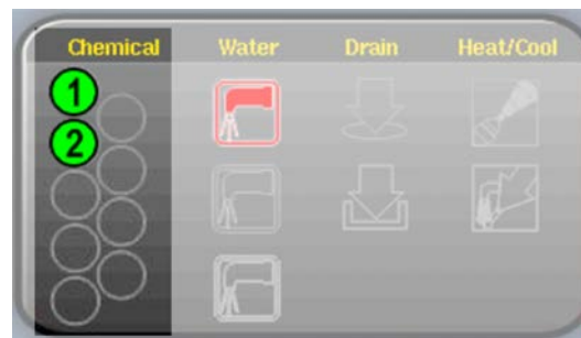
Figure 13. Chemicals from Valves 1 and 2 Injecting
