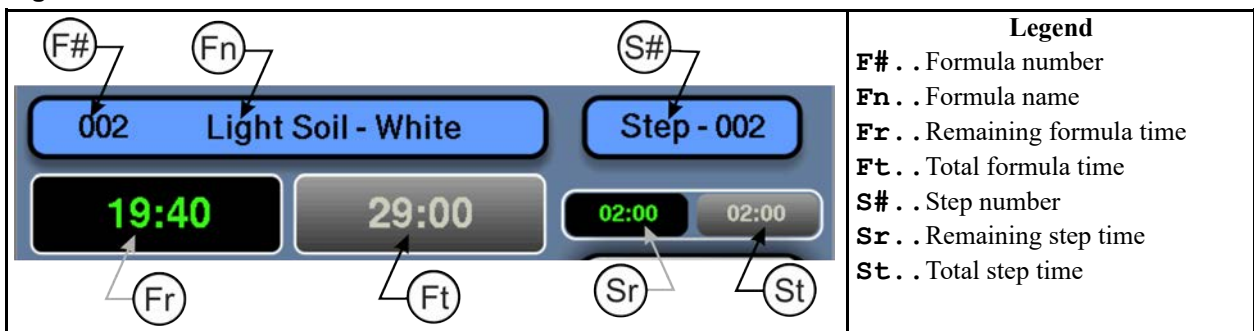
Figure 11. The Names and the Timers Area
