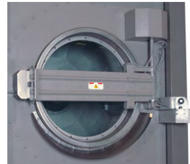
Figure 6. Hydraulically-operated Automatic Door
