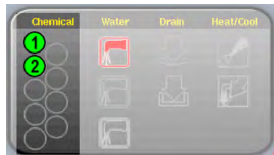
Figure 13. Chemicals from Valves 1 and 2 Injecting
