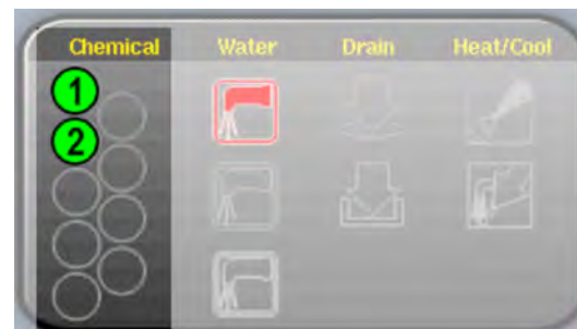
Figure 12. Chemicals from Valves 1 and 2 Injecting
