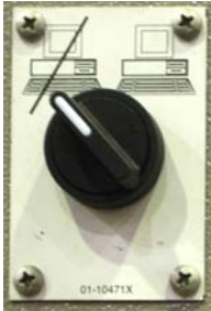
Figure 6: Mildata/Local Selector switch
