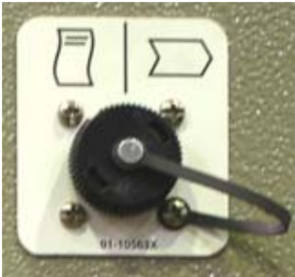
Figure 2: Serial Connection for Data Transfer
