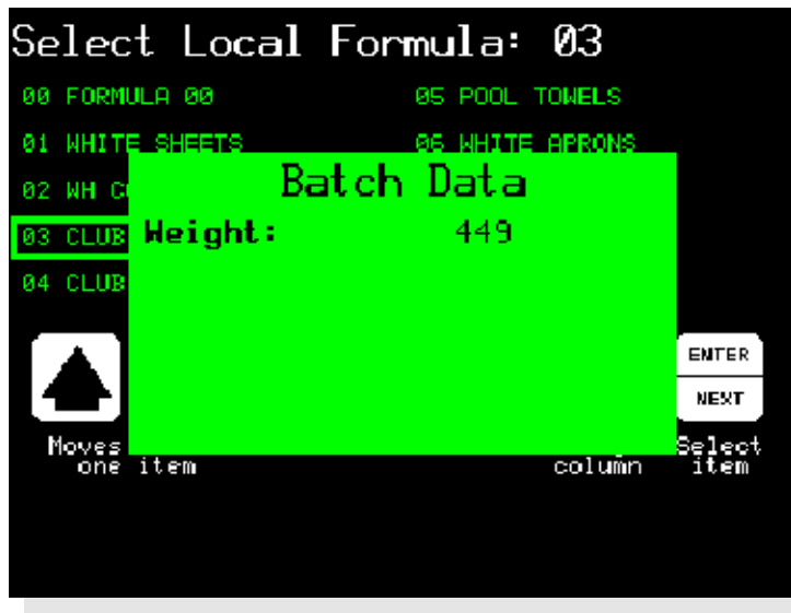
Figure 11: Entering Load Weight for Metered Water
