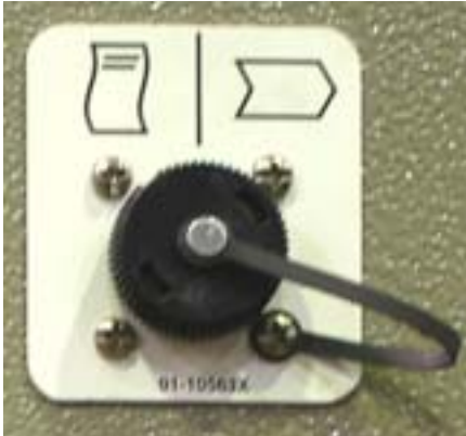
Figure 2: Serial Connection for Data Transfer
