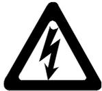
**SHOCK HAZARD**—High voltage electricity is present in electrical devices on this machine whenever external power is supplied, even if all power switches are off. Contact with high voltage electricity will kill or seriously injure you.
