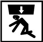
**CRUSH HAZARD**—Bucket may slowly descend even with power off or three-wire disabled, crushing anyone under it.
