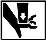
**CRUSH, ENTANGLE AND SEVER HAZARDS**—Contact with the turning cylinder can crush your limbs. Contact with the goods being processed can cause the goods to wrap around your body or limbs and dismember you. The turning cylinder and goods are normally isolated by the locked cylinder door.
