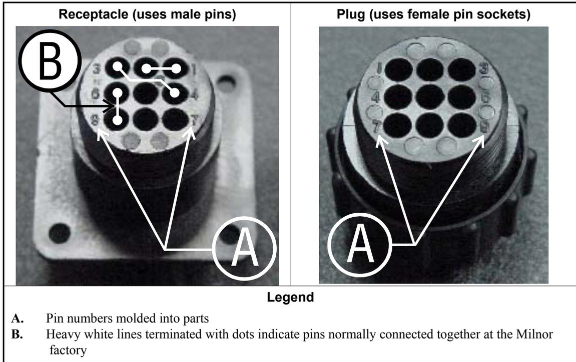
Table 1: External Serial Link Pin Assignments
