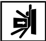
**STRIKE / CRUSH HAZARD**—A traveling machine such as a shuttle can strike, crush, or entrap you if you enter its path. Traveling machines or their components can move automatically in any direction. Placing a system machine on line by energizing the machine control may immediately summon a shuttle or other traveling machine.
