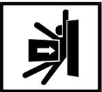
**CRUSH HAZARD**—The machine can crush your body or limbs if you are caught between the tilting housing and a stationary object.
