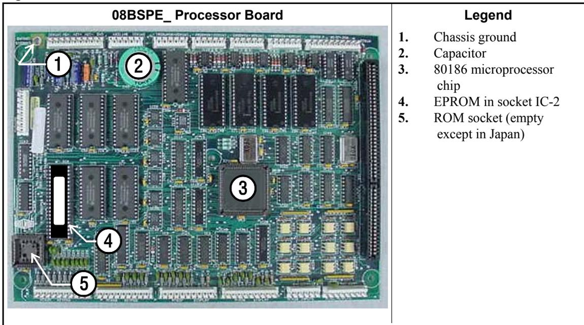
Figure 8: 80186 Processor Board
