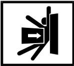
**STRIKE / CRUSH HAZARD**—Machines in the washing system move automatically and will strike or crush anyone in their path.
