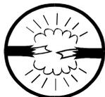
**COMPONENT DAMAGE HAZARD**—Board components will burn out, requiring board replacement if devices driven by inject signals do not meet the electrical specifications. (Pumps generally draw a higher current and will burn out board components.)
