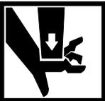
**CRUSH HAZARD**—Machine can crush body parts caught in gaps around shell front and at rear of machine that close due to vibration and tilting.
