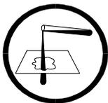
**MACHINE DAMAGE HAZARD**—Stainless steel surfaces can corrode if chemicals (e.g., bleach) dry on them, leaving residue. Rubber and plastic components (other than plastic cups) can deteriorate from exposure to chemical concentrates.
