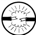
**COMPONENT DAMAGE HAZARD**—Devices driven by injection output signals which exceed electrical specifications will burn out board components, requiring board replacement. (Pumps generally draw a higher current and will burn out board components.)
