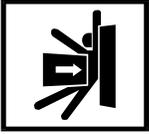
**STRIKE AND CRUSH HAZARDS**—The moving door can strike you or crush or pinch your limbs if caught between the door and machine.
