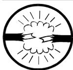
**COMPONENT DAMAGE HAZARD**—Interpret relay contacts will fail, requiring relay replacement if devices exceed the specified current load.
