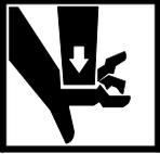
**CRUSH HAZARD**—Machine can crush body parts caught in gaps around shell front that close due to push down/release motion and machine vibration.
