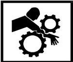
**ENTANGLE AND SEVER HAZARDS**—Contact with moving components normally isolated by guards, covers, and panels can entangle you and crush your limbs. These components move automatically.
