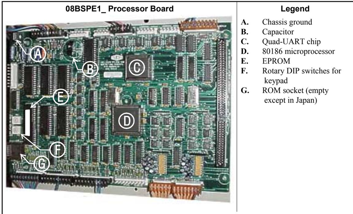
Figure 9: 08BSPE2\_ 80186 Processor Board
