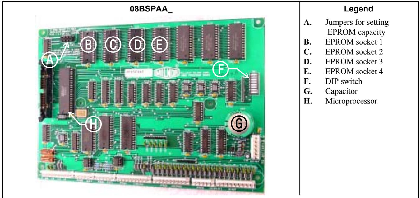
Figure 3: Where to Check Processor Board Voltages
