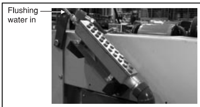
FIGURE 4 (MSSM0262CE) 15-Port Pumped Chemical Inlet
