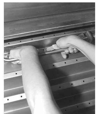
FIGURE 3 (MSOP0268AE) Releasing Top Door Locks
