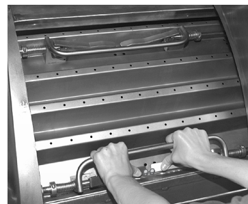
FIGURE 4 (MSOP0268AE) Release the Bottom Door Locks
