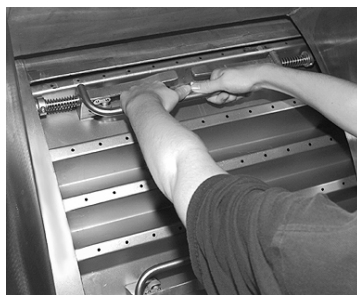
FIGURE 6 (MSOP0268AE) Pull Top Handle Up
