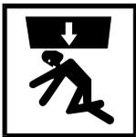
**CRUSH HAZARD**—The pre-press tamper or main press bell may slowly descend even with power off or three-wire disabled, crushing anyone under it.
