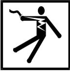
**SHOCK HAZARD**—Contact with high voltage electricity will kill or seriously injure you. High voltage electricity is present in electrical devices on this machine whenever external power is supplied, even if power switches are off.
