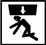
**CRUSH HAZARD**—Descending press main bell or pre-press tamper will strike and/or crush anyone under it. Main bell and tamper can descend with power on or off.
