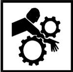
**CRUSH HAZARD—**Devices in and above the press move without warning and can entangle, crush, or sever limbs on contact.
