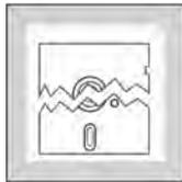
▶ Do not assume that the switch is right side up. Always reference the labels (**OFF, ON, 1, 2, etc.**) **printed on the switch** when setting DIP switches.
