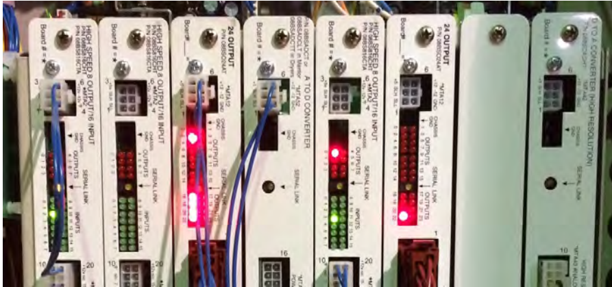
Figure 39. I/O Boards on a MilTouch-EX™ Machine
