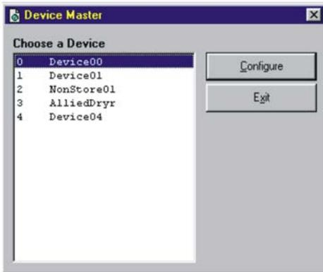
To display the **Device Configuration** screen (Figure 37, page 46), click the mouse on the **Configure** button in the **Device Selection** window. To exit the **Device Selection** menu without making any changes, click on the **Exit** button.
