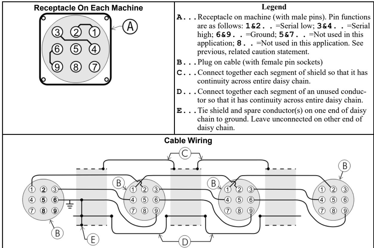
The internal connections on each receptacle (machine) between pins 1 and 2, 3 and 4, and 6 and 9 make it easier to wire the cable because it is not necessary to jumper these pins together on the cable. However, this also means that every plug on the daisy chain must be plugged into a receptacle. Otherwise, the serial low, serial high, and ground conductors will not have continuity across the entire daisy chain and some machines will not receive data.
