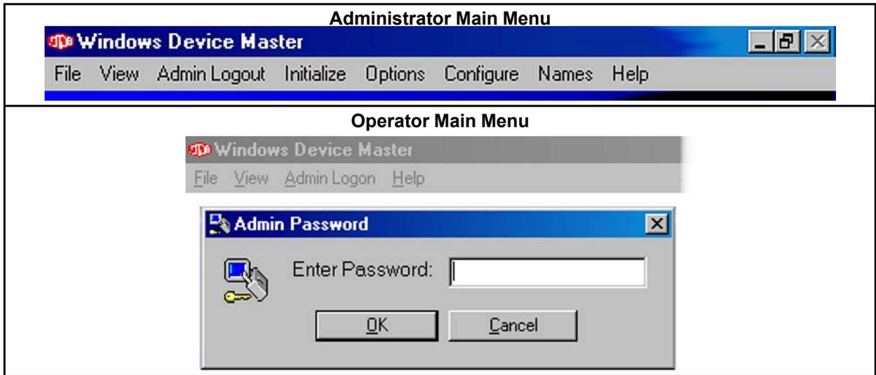
Any menu selection which is used to modify configuration data cannot be implemented while the Device Master controller is in operation. In those cases, the user will first be prompted by a message box, as shown in Figure 9, page 7, to disable the three wire circuit before access to that selection is allowed.
