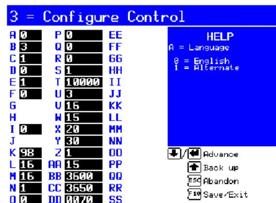
**2.1.5.1. When is Configuring Required?**—Your machine was configured when it was tested at the factory, but you should verify that all decisions match your hardware and preferences before putting the machine in service. Make a copy of your machine configuration for future reference.
