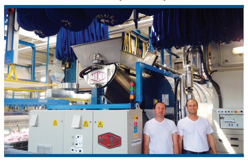
After 23 years of continued use, LSG Laundry recently replaced their GI CBW® tunnel with a new 8-mod 50 kg PBW™ tunnel, 40-bar single stage press, and three pass-through dryers. The new system features touchscreen Mentor® control, live camera feed from the load chute, RecircONE® pump, and infrared sensors in the dryers. Their new 8-mod PBW™ tunnel has allowed LSG Laundry to enjoy increased productivity and excellent wash quality.
