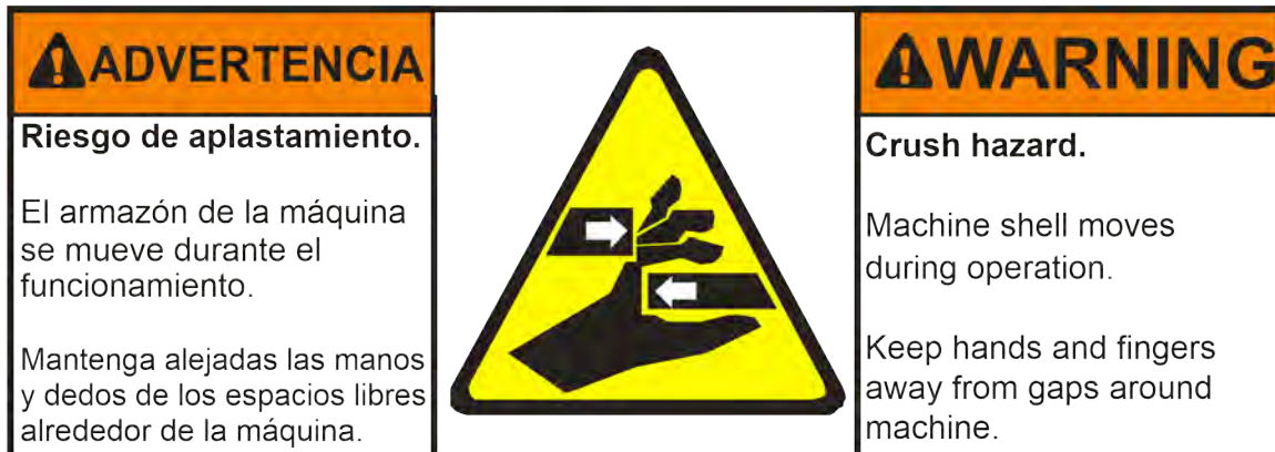
Figure 4. External Mechanical Hazards—Closing Gaps On Machine
