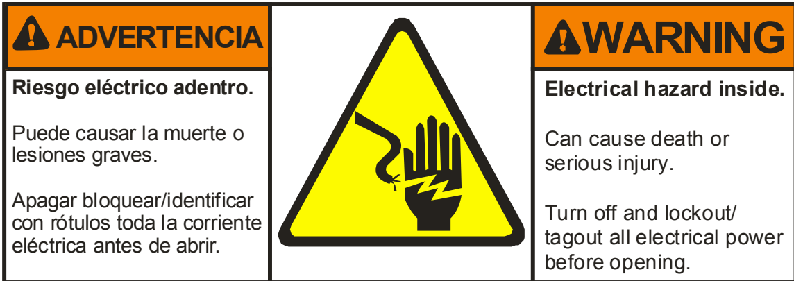
Figure 1: Internal Electrical and Mechanical Hazards—Electricity
