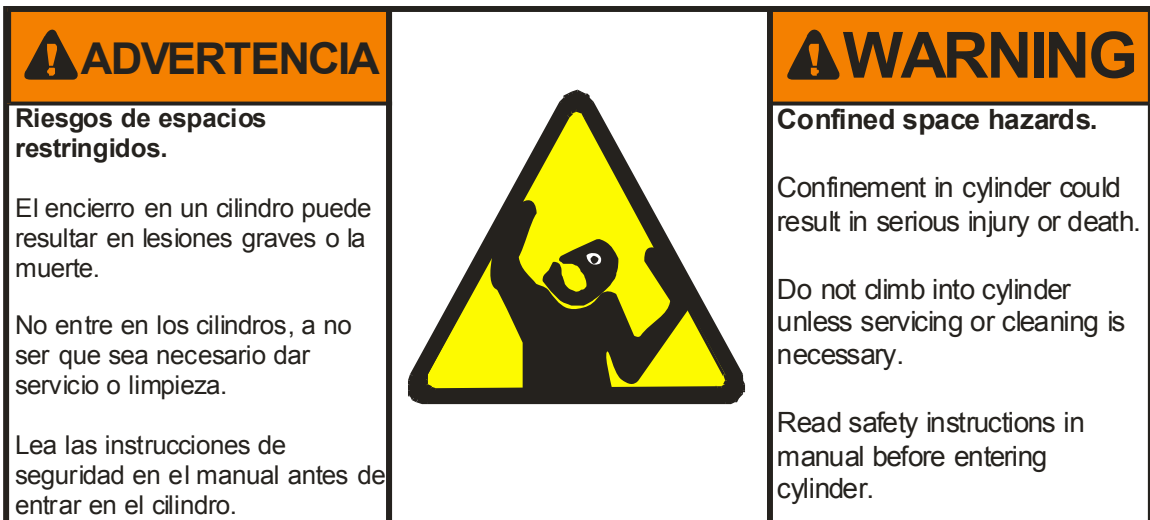
Figure 8: Cylinder and Processing Hazards—Confined Space
