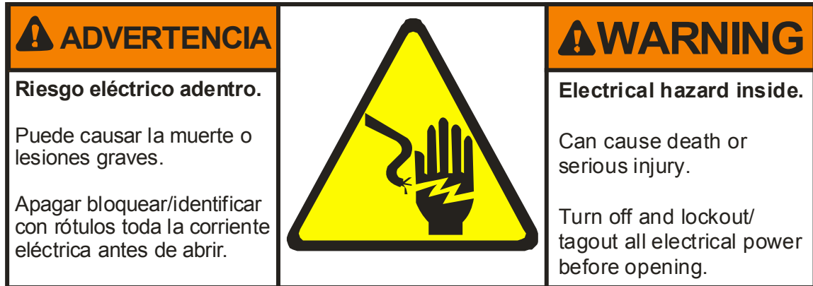
Figure 1: Internal Electrical and Mechanical Hazards—Electricity
