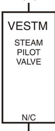
Figure 19: Electrically Operated Valve (VE)
