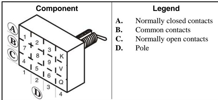
Figure 27: Switch with Replaceable Contact Blocks
