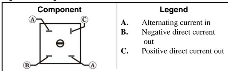
**WC=Wiring Connector**—A coupling device for joining two cables or connecting a cable to an electronic circuit or piece of equipment. Connectors are male or female, according to whether they plug into or receive the mating connector.
