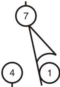
Figure 16: Pressure Switch (SP)
