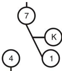
Figure 14: Level Switch (SL)
