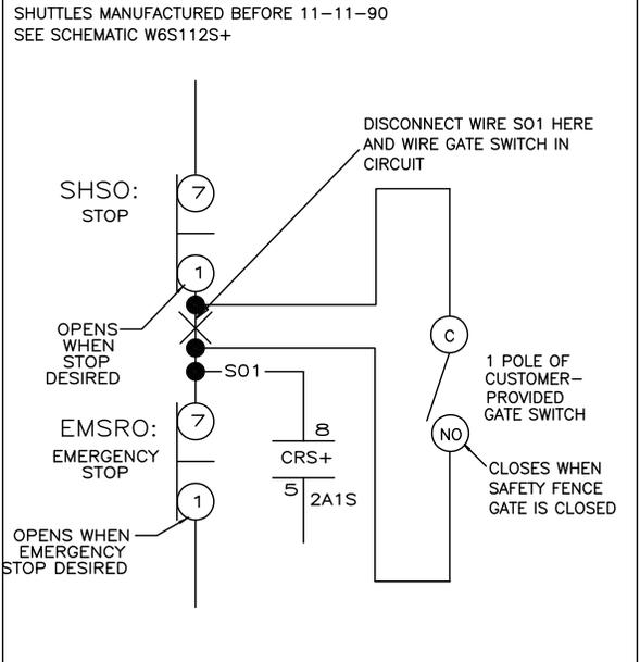
SAFETY FENCE GATE WIRING FOR ALL 2 STAGE PRESSES
