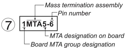
An MTA is a connection on an electronic circuit board. The notes and the tag page locate the appropriate board.
