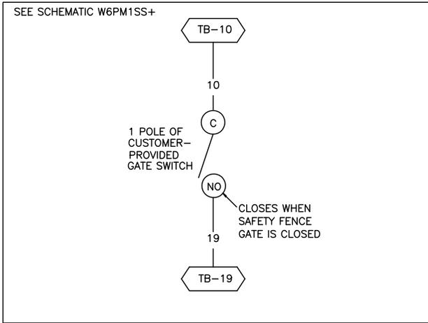
SAFETY FENCE GATE WIRING FOR ALL CENTRIFUGAL EXTRACTOR
