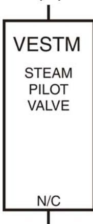
Figure 19: Electrically Operated Valve (VE)
