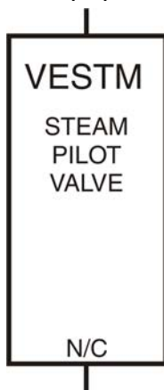
Figure 19: Electrically Operated Valve (VE)
