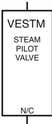
Figure 19: Electrically Operated Valve (VE)
